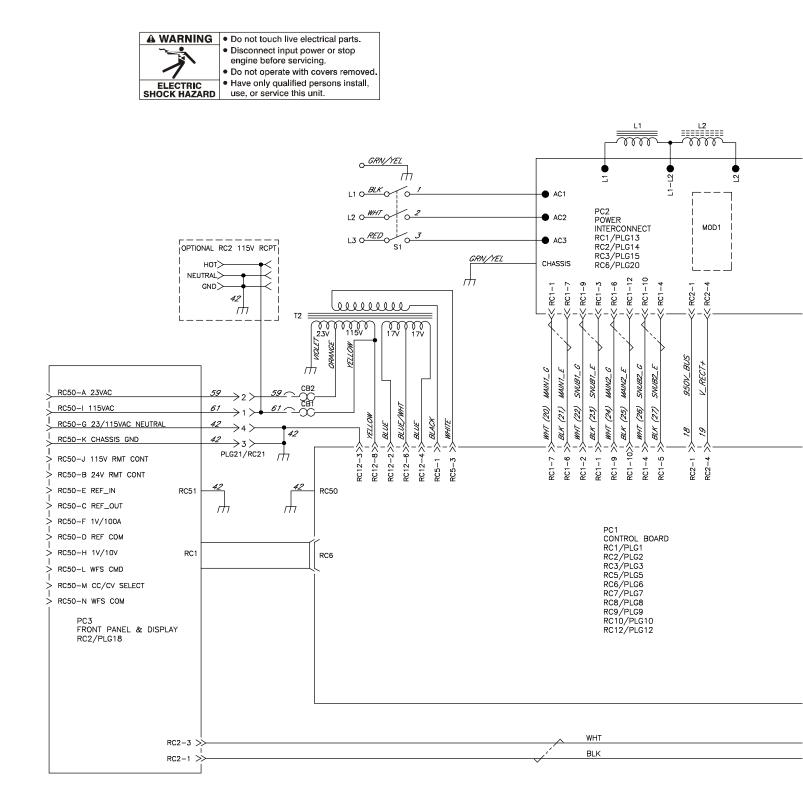
Figure 10-1. Circuit for Invision 352 MPa (208–575 Volt) Eff. w/Serial No. MA021803A thru MB380100A
