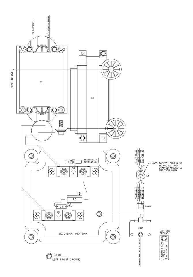
Figure 10-16. Wiring Diagram for Invision 352 MPa Eff. w/Serial No. MF254023U And Following (2 of 2) TM-246193 Page 98 Invision 352 MPa
