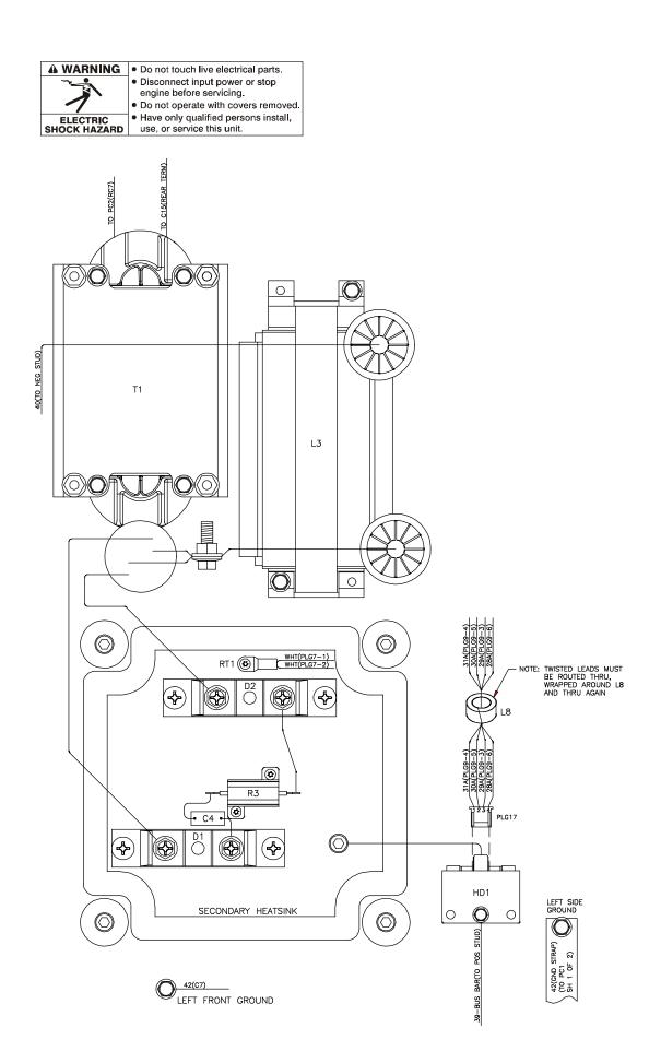
Figure 10-14. Wiring Diagram for Invision 352 MPa Eff. w/Serial No. ME224001U Thru MF254022U (2 of 2)
