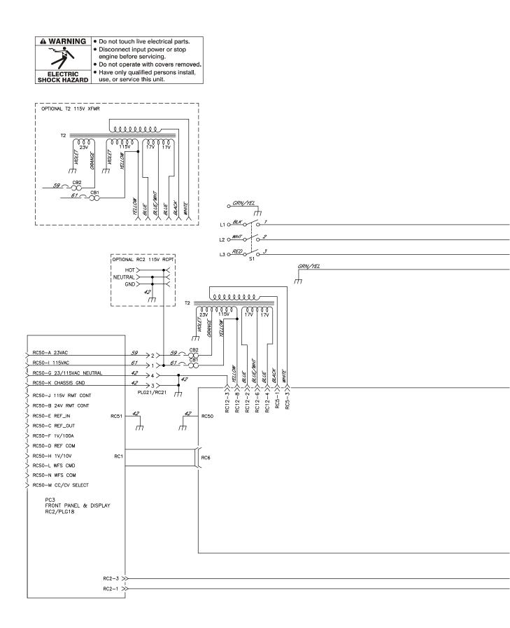
Figure 10-3. Circuit for Invision 352 MPa (208–575 Volt) Eff. w/Serial No. MB520506A Thru ME224000U
