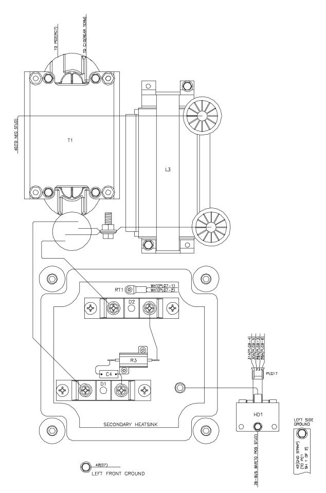
Figure 10-8. Wiring Diagram for Invision 352 MPa Eff. w/Serial No. MA021803A And Following (2 of 2)
