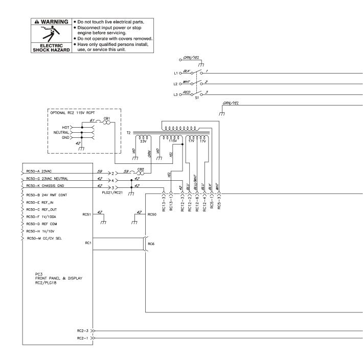
Figure 10-5. Circuit for Invision 352 MPa (208-575 Volt) Eff. w/Serial No. MF254023U Thru MF344114U
