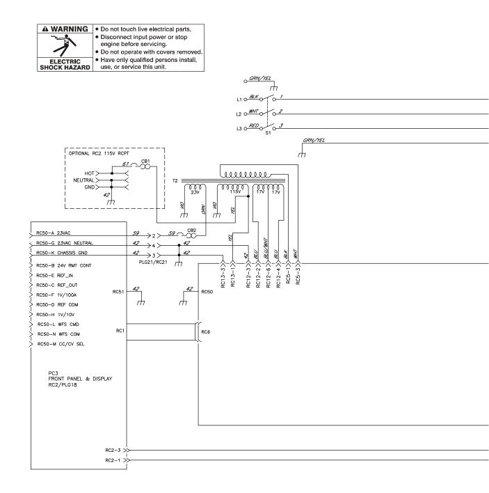
Figure 10-6. Circuit for Invision 352 MPa (208-575 Volt) Eff. w/Serial No. MF344115U And Following
