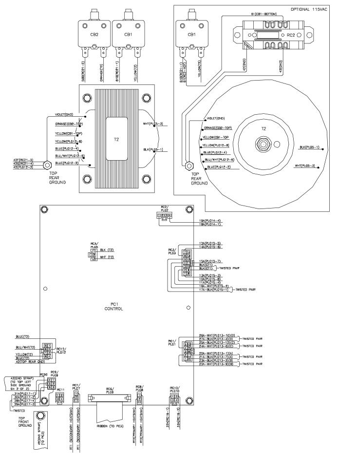
Figure 10-7. Wiring Diagram for Invision 352 MPa Eff. w/Serial No. MA021803A And Following (1 of 2)
