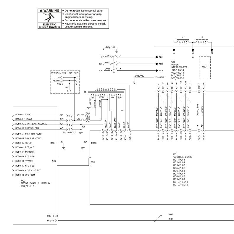
Figure 10-2. Circuit for Invision 352 MPa (208–575 Volt) Eff. w/Serial No. MB380101A thru MB520505A
