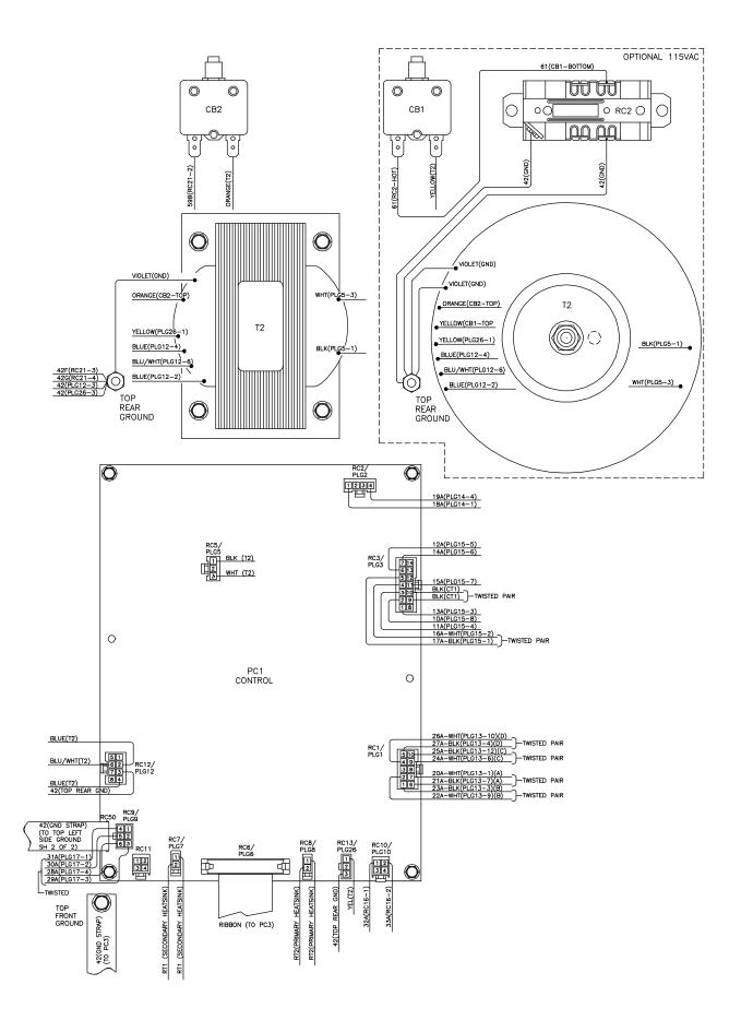
Figure 10-15. Wiring Diagram for Invision 352 MPa Eff. w/Serial No. MF254023U And Following (1 of 2) TM-246193 Page 96
