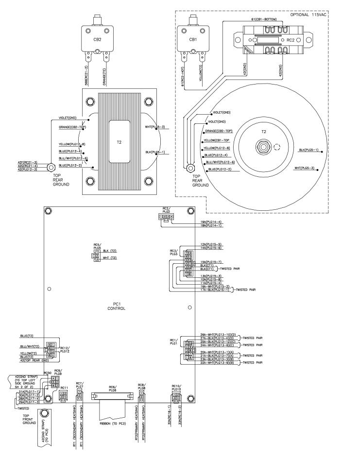
Figure 10-13. Wiring Diagram for Invision 352 MPa Eff. w/Serial No. ME224001U Thru MF254022U (1 of 2)
